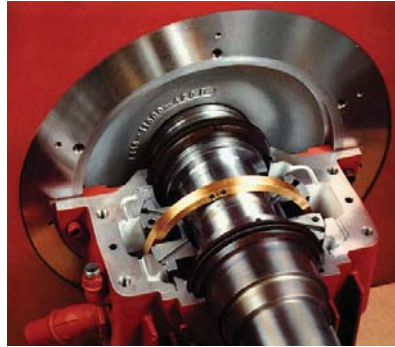
Photo 3. Typical sleeve bearing arrangement with the top half of the bearing removed for inspection.
