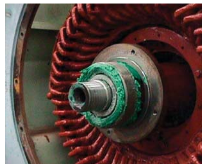
Photo 1. This bearing was relubricated with an excessive quantity of grease.
