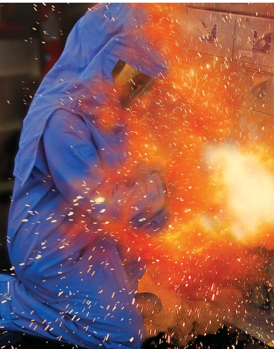
Photo 1. An arc flash can generate an electric arc with a temperature of 35,000°F.
