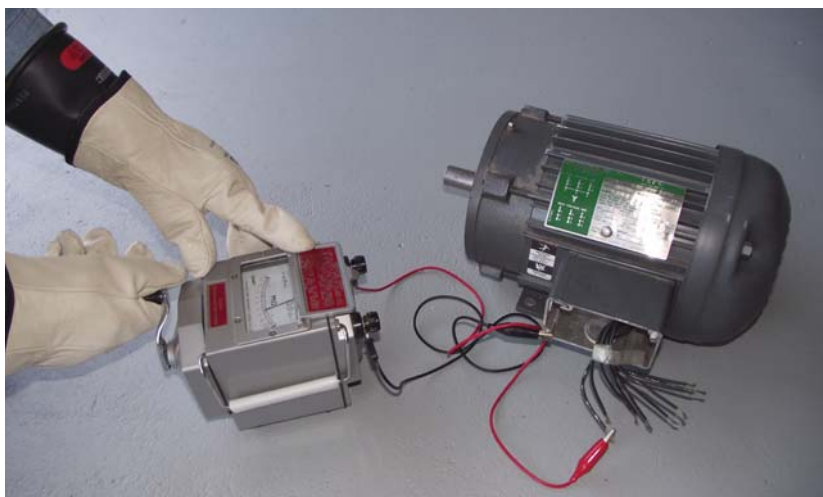
Fig. 3a. This megohmmeter requires hand cranking of an internal generator for the duration of the test to provide the test voltage. An analog scale on the face provides the resistance in megohms.
