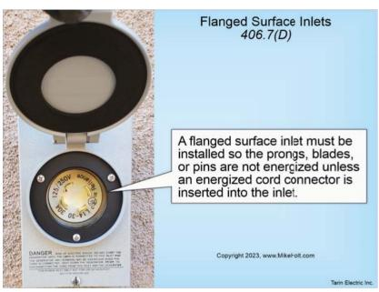
Fig. 3. The requirements for the installation of a flanged surface inlet are found in Sec. 406.(D).
