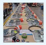
We do all pre-assembly in our warehouse including brackets with attached junction boxes, devices and rings, as well as cutting MC cable.
