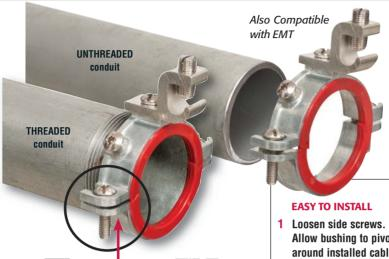
Get convenience and time-savings with Arlington's 550 series SPLIT grounding bushings. The split allows the addition of a bushing AFTER conductors are installed in threaded or unthreaded Rigid/IMC conduit. Great for tight spaces!
