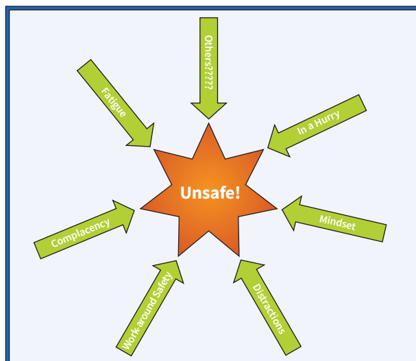
Fig. 2. Incidents are typically caused by a combination of issues. Removing any one of several potential issues may help prevent an incident. Proper job planning and job briefings should identify and eliminate hazards.
