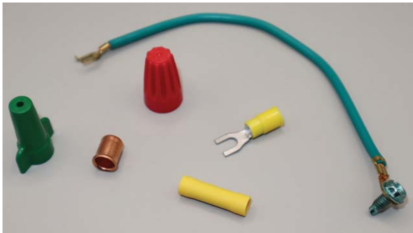
Photo 1. Listed pressure connectors are often used for bonding connections. Typical connectors are twist-on type connectors and tool-crimped connectors. At left is a green twist-on connector with a hole in the top to allow pushing through of a solid equipment grounding conductor to bond to the wiring device. The green bonding jumper at the top is prefabricated with listed tool-crimp connectors at each end. The red twist-on connector can be used for grounding and bonding applications. The tool-applied crimps (bottom center) are listed for stranded conductors only.
