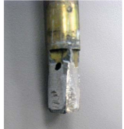
Photo 7. Care must be taken not to rack too hard.
