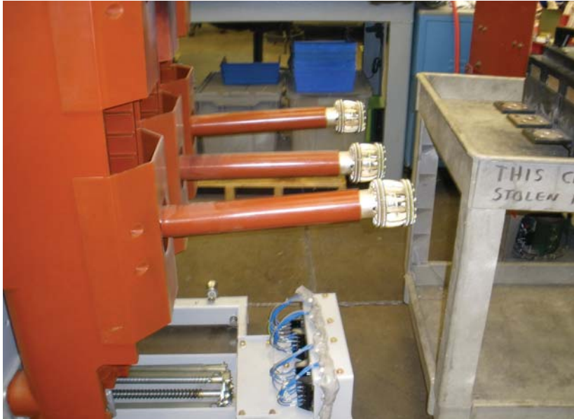
Photo 5. Note how this circuit breaker has some bent bus connection arms
