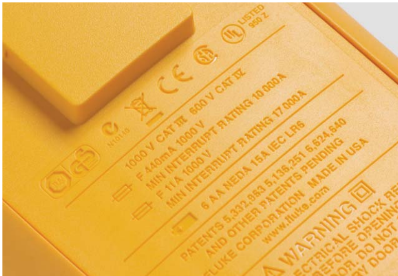
Photo 1. Check for appropriate CAT ratings, IP codes, and independent verification symbols to be sure the meter you select has been tested by an independent lab and is safe for your measurements.
