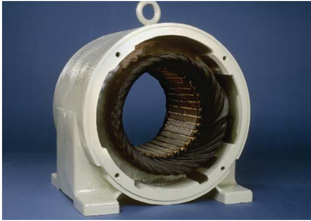
Photo 2. Excessive overheating failure caused by an overload condition.
