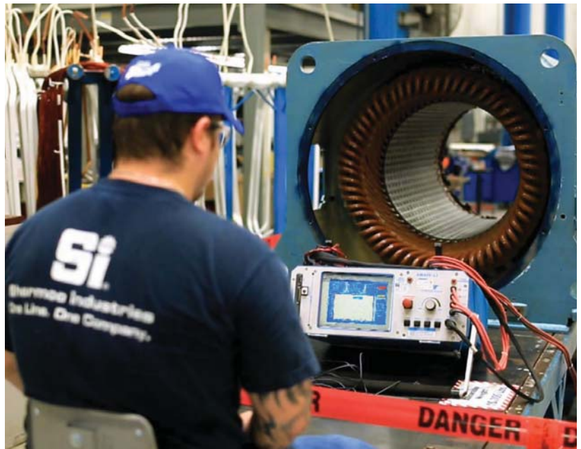
For safely testing motors, caution tape establishes a safe perimeter around moving parts.
